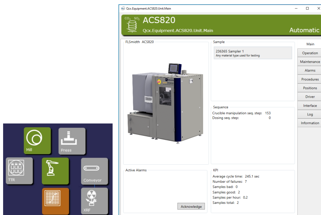
Figure 11. Status monitoring. The basic system indicates status via colour-changing symbols (left). More advanced systems include detailed faceplates (right).
