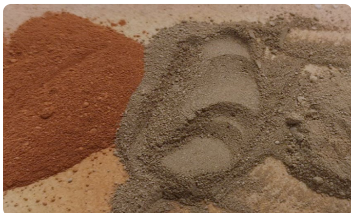
Colour control with flash calciner Comparison with and without colour control
