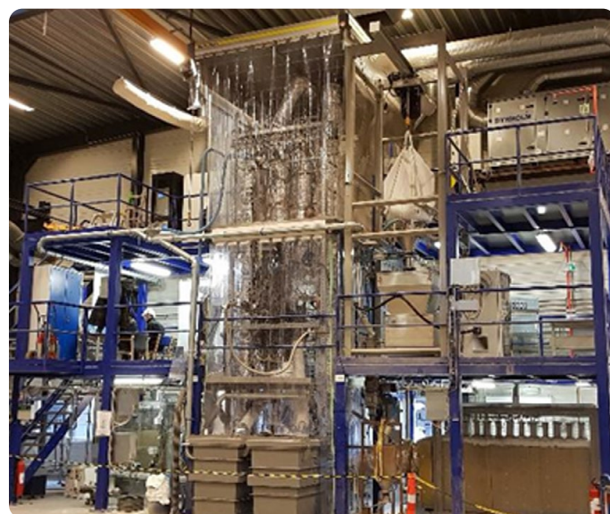
Pilot Installation for SCM pyroprocessing - At Fuller Technologies' R&D Center Dania, Denmark
