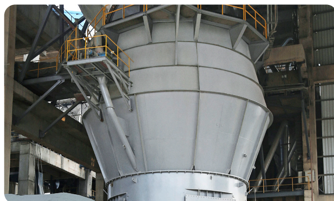
Example of ROKSH separator for optimum cement product quality.
