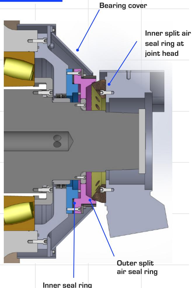
The new split design eliminates the need to disassemble the joint head to remove the seal, allowing easy replacement. The seal air gap can also easily be adjusted by adding shims. The result is improved sealing performance and increased operational reliability.
