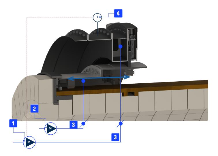
The outlet cooling system is separated into two independent systems – one for the kiln shell and nose ring cooling and one for the graphite cooling. The graphite cooling is designed to maintain the temperature of the graphite blocks below oxidization temperature and secures the flatness of the flange module.
