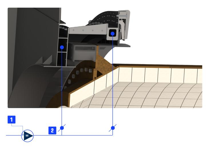
The inlet cooling system consists of a fan and a closed isolated ducting system to cool vital sealing components. The cooling air is distributed to the rear flange and the air cooling chamber attached to the kiln riser. The air will escape into the atmosphere.
