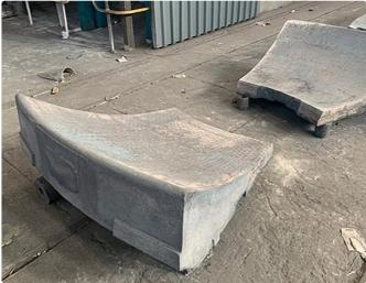
OK Pro+ wear liners are currently available for rollers and tables of all  $OK^{TM}$  raw mills and most OK cement mills with full roller segments.
