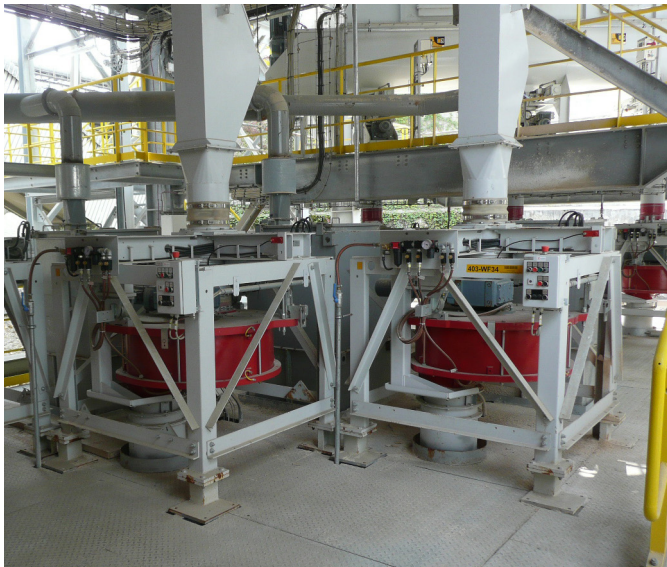
Pfister® FRW blending installation at the finish mill of a cement plant in Germany.
