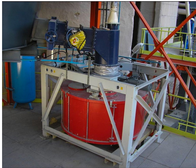
Kiln feed installation at a clinker production line in Romania.
