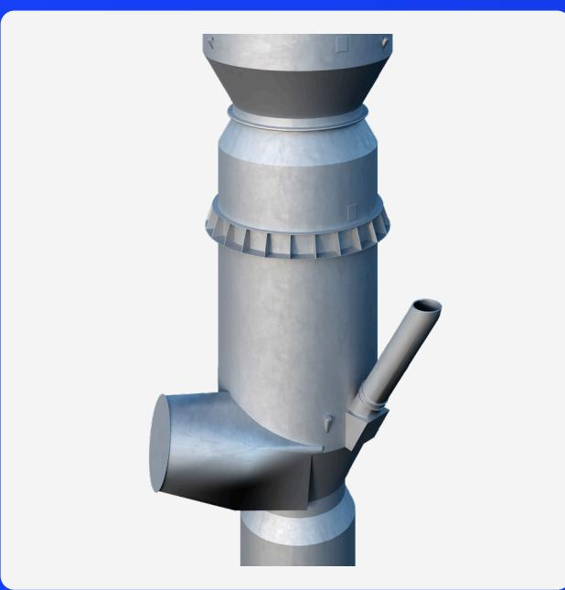
The unique design of the lower calciner optimises dispersion of the raw meal into the gas stream.
