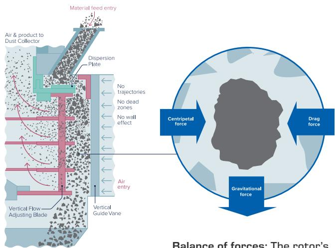
**Balance of forces:** The rotor's speed directly affects the centripetal force. The amount of airflow affects the drag force
