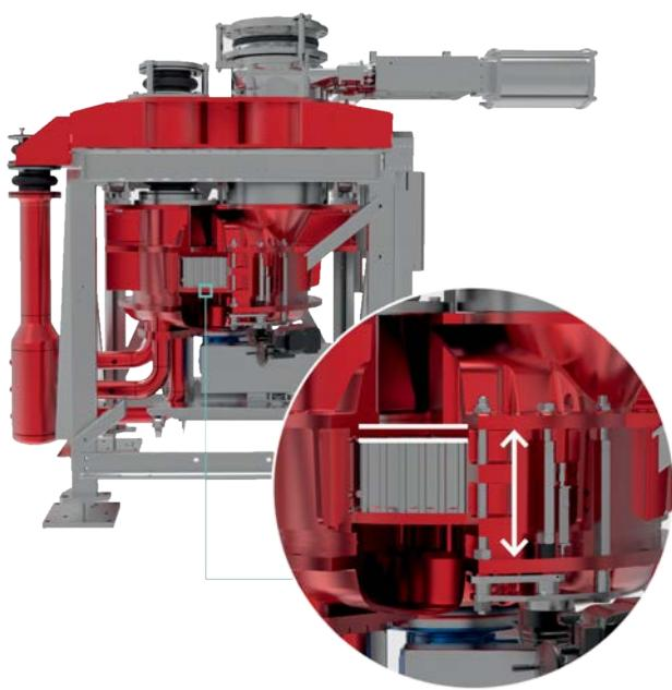
Getting the gap width right in your DRW rotor weighfeeder is crucial for smooth operation. Too large or too small a gap and you risk blockages, reduced dosing accuracy, and high levels of wear and tear. Enter the Pfister AutoGAP 2.0, which automatically adjusts and controls the upper gap width to ensure best possible performance.
