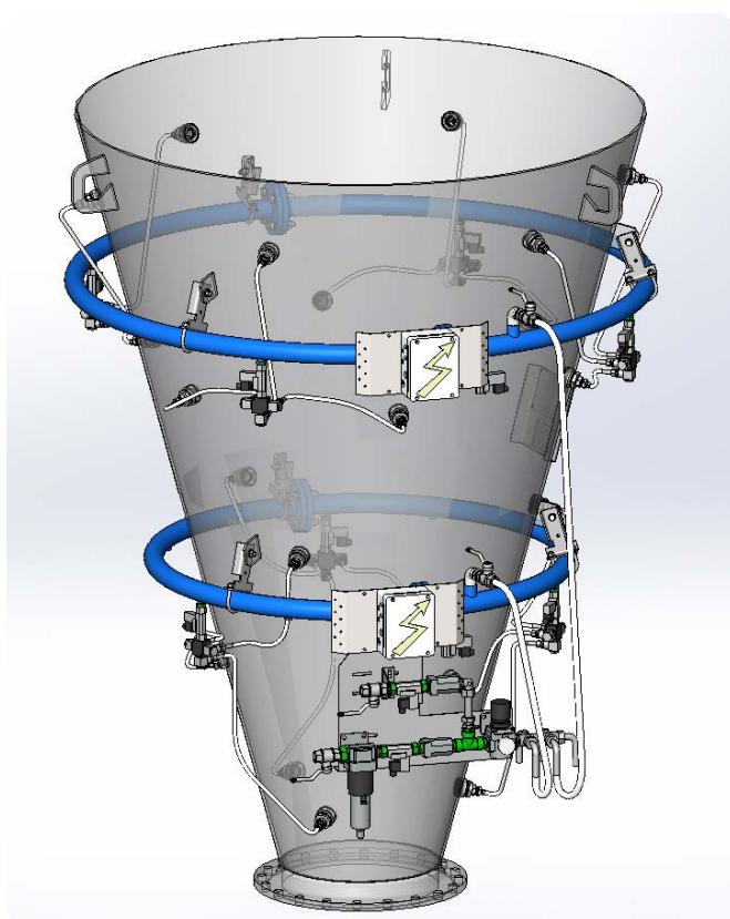
Traditional rotor weighfeeder operations rely on fixed aeration intervals. But these don't account for changing flow behaviour between the prehopper and silo bottom. Ultimately, you can end up using too much air and wasting money, or not enough, and losing productivity.
