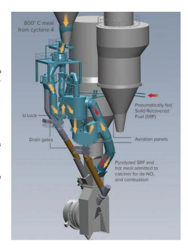
Re-burning reactions utilizing SRF pyrolysis gases to convert NO into free  $\rm N_2$  in the reduction zone prior to mixing with preheated combustion air in the calciner.
