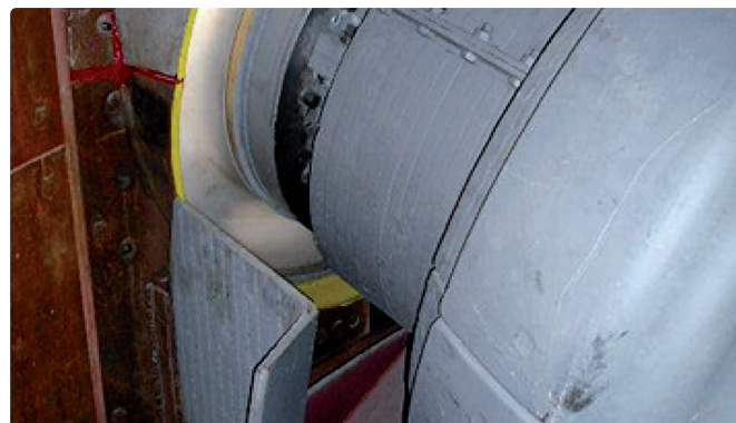
Flexible seal between housing and roller
