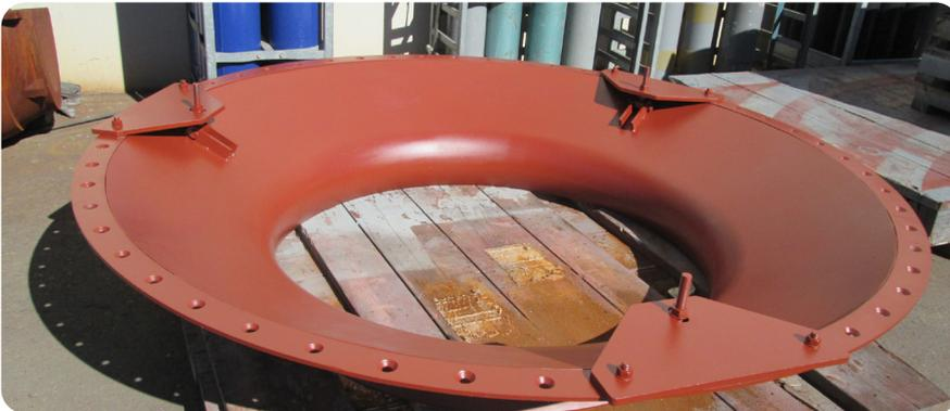
Tool for easy adjustment of inlet cone
