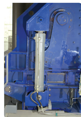
Hydraulic cylinder to open top part of crusher
