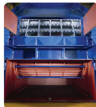
Opening for dismantling breaker plates and outlet grate adjustment
