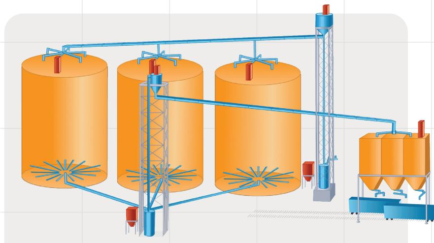
Airlift™ vertical conveyors and Airslide® gravity conveying systems convey alumina at a net rate of 750 mtph in a major western United States facility
