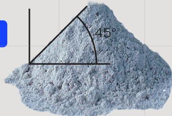
All dry bulk material has a natural angle of repose, often in excess of 45°.
