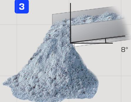
With fluidization, gravity flow can be achieved at a greatly reduced slope - of 8° or less.
