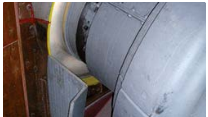
Flexible seal between housing and roller
